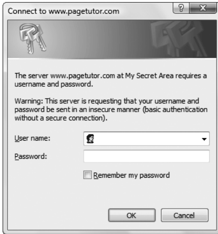
Figure 17-5. Internet Explorer shows this password prompt when a page requiring authentication is requested.
